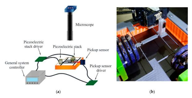
**Figure 13.** Experimental setup to obtain the displacement of the XY microdisplacement platform, (**a**) schematic diagram. (**b**) Measurement of displacement by the pickup sensor.
