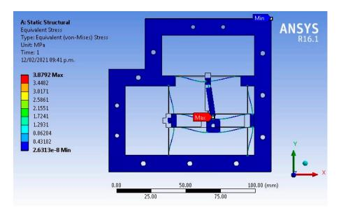
Figure 11. Maximum equivalent stress when forces are applied to each axis simultaneously.
