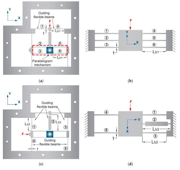
$L_{b2}$  and  $L_{b3}$  are the corresponding lengths of the beams.
