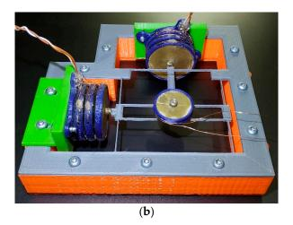
Figure 7. (a) Scheme diagram of the biaxial positioner, and (b) its implementation with PLA.
