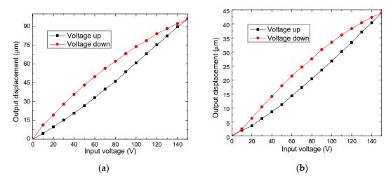
Figure 3. Deformation for piezo buzzers described in Table 2 and used for (a) X-axis and Y-axis, and (b) Z-axis displacements.
