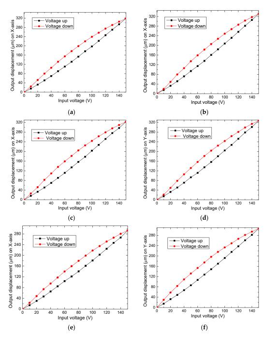
**Figure 14.** Output displacement on the X-axis and Y-axis, respectively, (**a**) and (**b**), for ABS. (**c**) and (**d**) for PETG. (**e**) and (**f**) for PLA.
