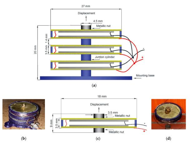
**Figure 4.** Buzzers stacks. (a) Schematic diagram of the piezo buzzer stack with six buzzers, for X and Y displacement axes. Transversal view, and (b) its implementation using a structure made with Polylactic Acid (PLA). (c) Schematic diagram of the piezo buzzer stack with two buzzers, for Z displacement axis, and (d) its implementation with a PLA support.
