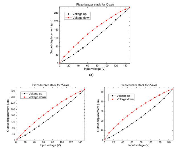
**Figure 5.** Graphs of output displacement versus applied voltage for piezo buzzer stacks for (**a**) X-axis, (**b**) Y-axis, and (**c**) Z-axis.
