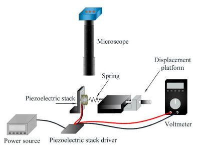
Figure 6. Experimental setup to register the blocking force generated by the piezoelectric actuators.
