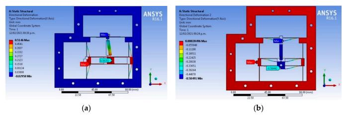
**Figure 9.** (a) X-axis and (b) Y-axis displacements obtained from the simulation in ANSYS. Results were achieved by applying a force only on the axis where displacement was measured.
