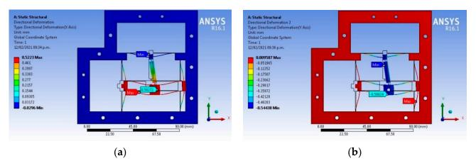
Figure 10. (a) The X-axis and (b) Y-axis displacements are obtained by applying the force in both axes at the same time.
