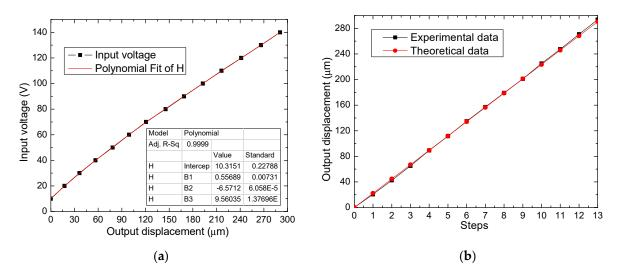
**Figure 15.** (a) Graph of the polynomial fitting. (b) Comparison of the linearized experimental and theoretical displacements given by the linearization model.
