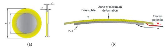
Figure 1. Piezo buzzer: (a) Dimensions A, B, C, and D are described in Table 2. (b) Transversal view, under deformation.
