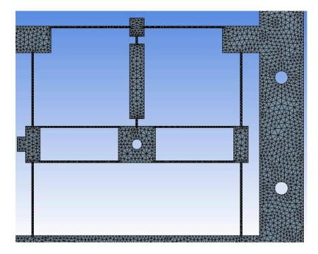
Figure 12. A zoom focused on the mash for the working platform of the micropositioner.
