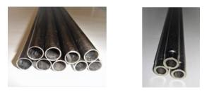
Fig. 4. Copper and 1018 steel tube with coating
