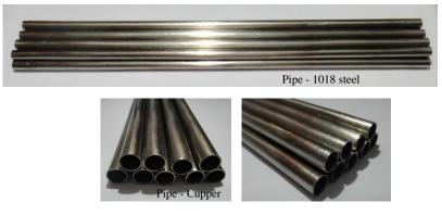
Fig. 6. Copper and 1018 steel pipe with Ni-P coating
