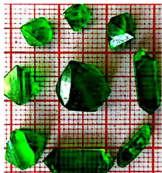
Figure 31. Anhydrous chiral potassium ferrioxalate crystals. Elemental analysis has confirmed the absence of hydrogen. Reproduced with permission from ref 412. Copyright 2012 Elsevier B.V.
