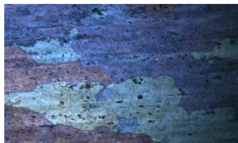
**Fig. 2** Aluminum 7075 (20X) with almost any precipitation
