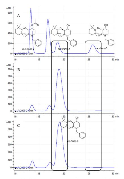
**Figure 3.** (**A**) Chiral-HPLC chromatogram of the 2:1 mixture of both *rac-trans-***2** and *rac-trans-***3**. (**B**) Chiral-HPLC chromatogram of the CALB-catalyzed de-acylation reaction at 24 h. (**C**) Chiral-HPLC chromatogram of the CALB-catalyzed de-acylation reaction at 72 h.
