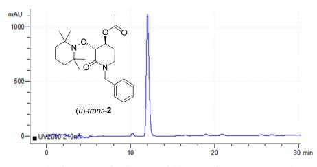
Figure 6. Chiral-HPLC acetylated compound (u)-trans-2 after 3 enzymatic resolutions.
