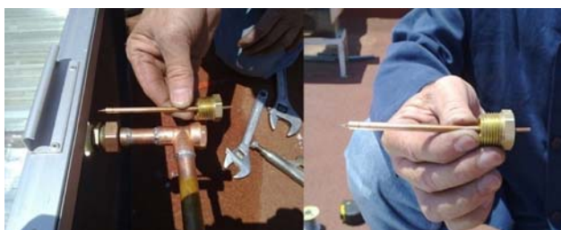
Fig. 8. Design of thermocouples well.
