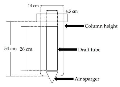
Figure 7. Scheme of an airlift bioreactor used for cell culture of A. pichinchensis.
