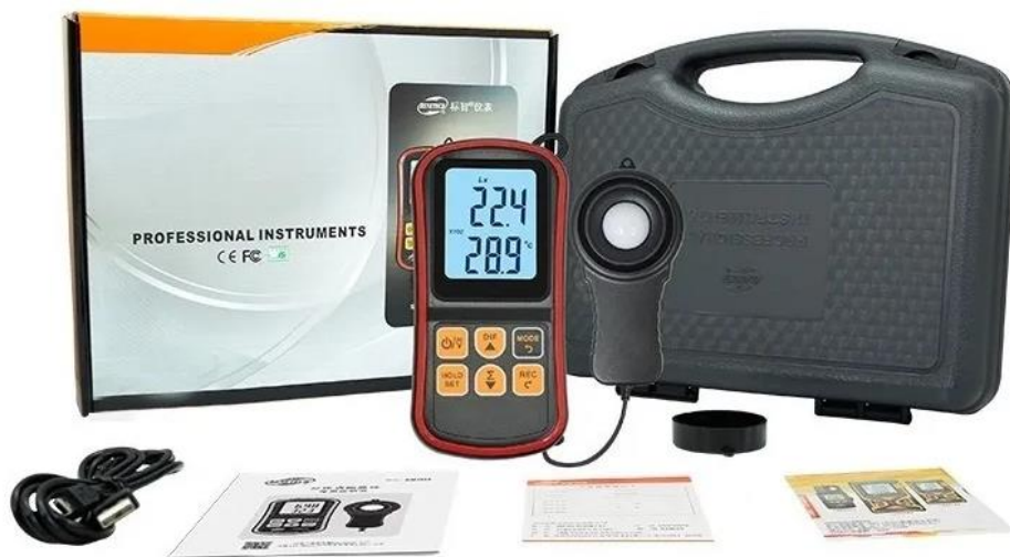
Figura 12. Luxómetro digital Benentech. Mod. Gm1020 Rango 0~200,000 Lux
